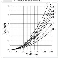
The diagram at the side shows the pressure drop curves for spools during normal usage. The fluid used is a mineral oil with a viscosity of 46 mm²/s at  $40^{\circ}\text{C}$ ; the tests have been carried out at a fluid temperature of  $40^{\circ}\text{C}$ . For higher flow rates than those in the diagram, the losses will be those expressed by the following formula:
